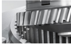
Power Skiving with integrated cutter sharpening
